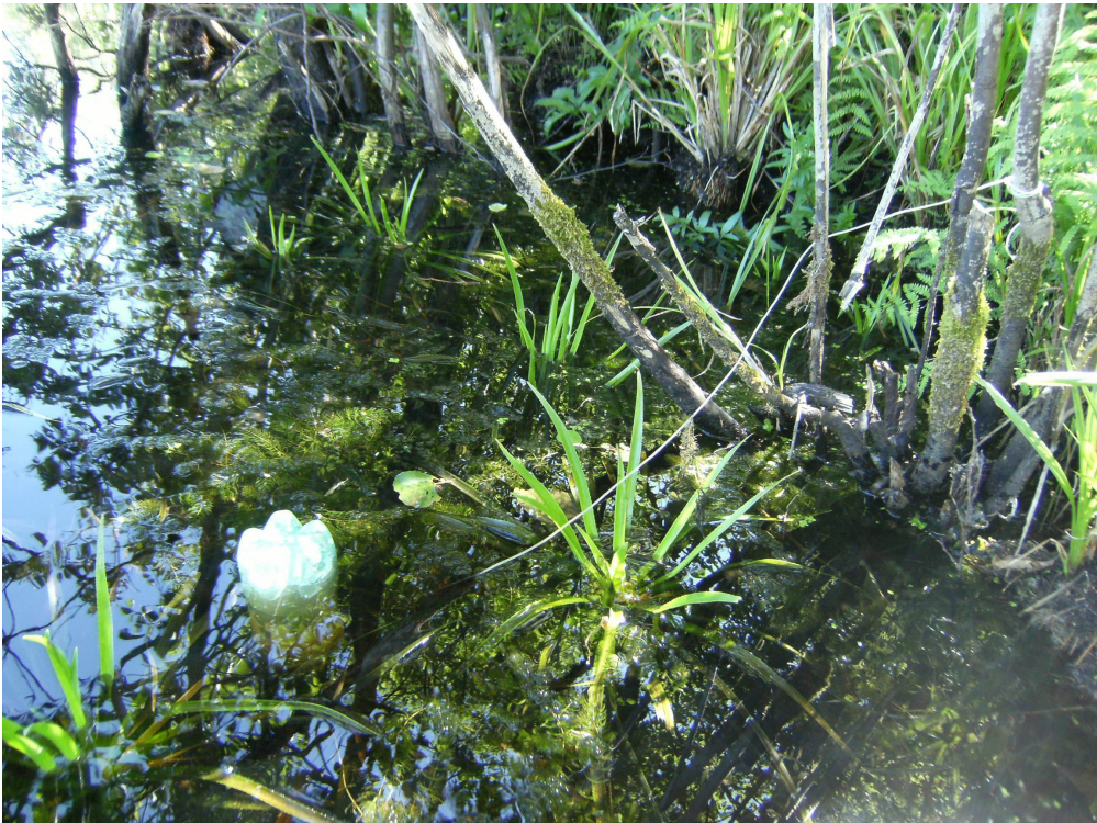
Figure 2. Funnel trap set near lake bank and fastened to a shrub by cord (Lake Glukhoye, July 2010).
